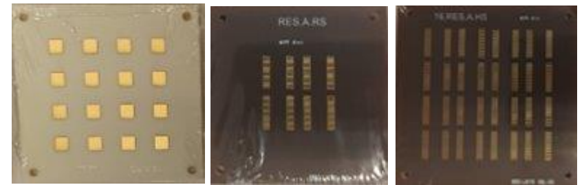
Manufactured layers of the antenna array (100x100 mm)
